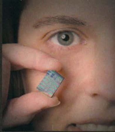
This is what's causing all the headaches. No, not IBM analysis engineer Tami Vogel but the small piece of silicon she's holding. With an area of 221mm 2 and consisting of 234 million transistors, Cell is the most powerful CPU designed for desktop and entertainment applications
